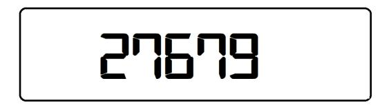
To read the meter, simply write down the number from left to right. In this case, the meter reading is 27679.
