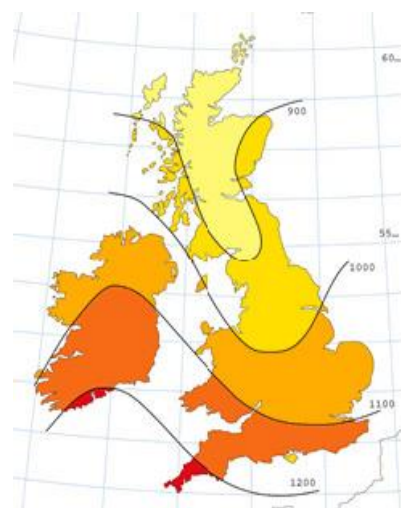
Figure 3: UK map showing average solar radiation for panel on 30° angle per year. Radiation is highest in areas shaded dark red, reducing to the lowest amount of radiation in areas shaded pale yellow. Taken from www.solar-trade.org.uk
